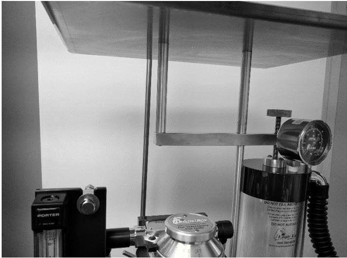
The **Bag Hanger Arm and IV Pole Combo** is mounted on the back of the vaporizer mounting plate. The **Mounting Screws** are installed from the front of the vaporizer plate, through the plate and into the **Bag Hanger Arm**.
